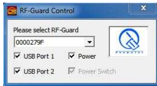
Fig. 4: GUI interface for interrupting the USB Ports and the power supply in the shielding box
