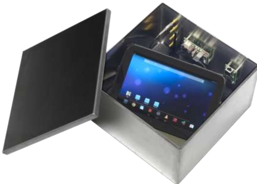
Figure 5: Shielding Box with a interior size of 30 x 30 x 17,5 cm
