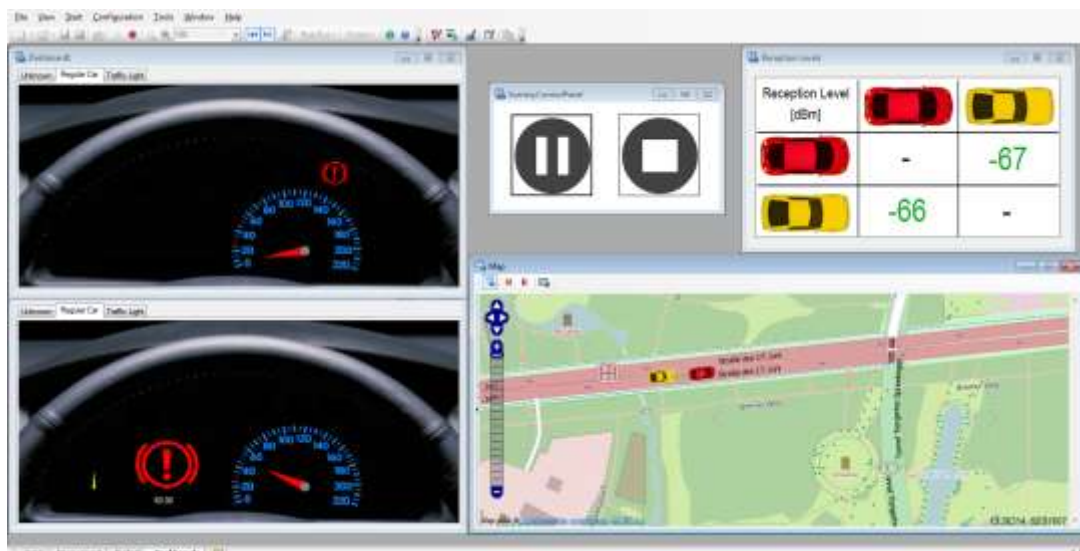
Figure 3: A traffic situation causing an emergency brake emulated with CANoe and QPER
