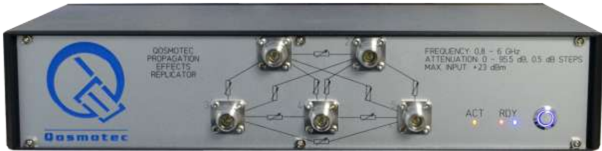
Figure 4: The QPER hardware with five ports and 10 attenuator controlled radio links
