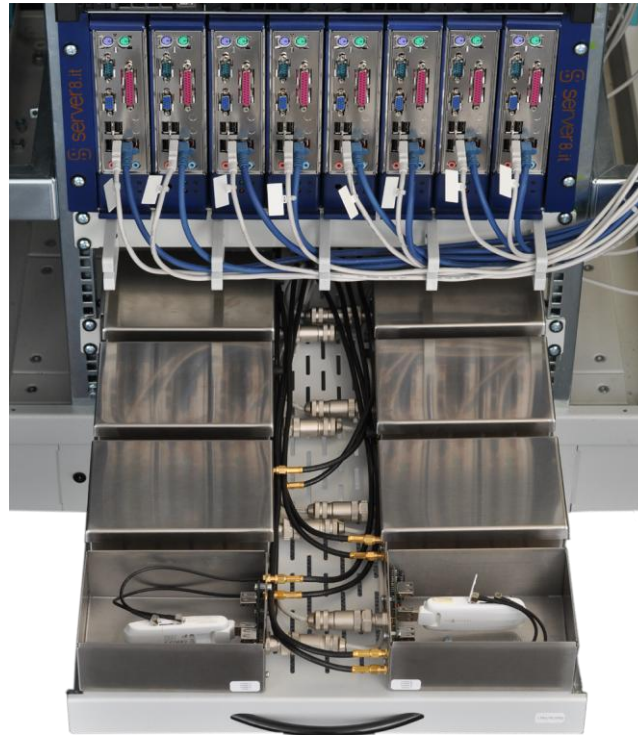
Figure 3: Rack setup for commercial UEs - 8 shielded boxes on a rack shelf, connected to 8 mobile control servers in a blade chassis
