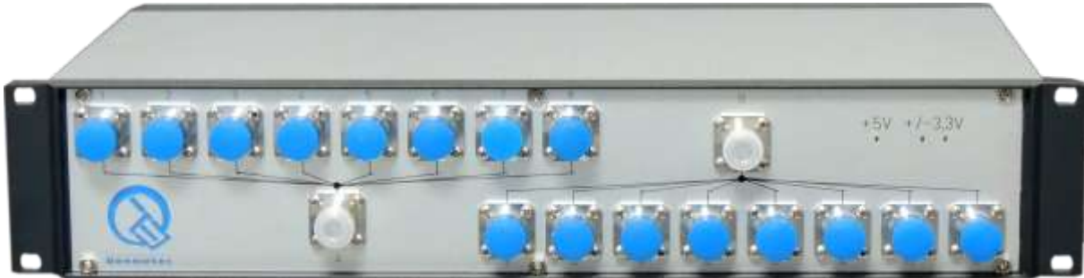
Figure 3: Switch System consisting of two 8:1 switches
