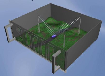
**QPER Test Bed** enables engineers to perform controlled mobile network test scenarios indoors without the need for a fully-fledged test lab. Based on Qosmotec's QPER/AIS technology, it allows to test UE and SIM-card functionality in a completely emulated mobile network. Thus, QPER Test Bed is the ideal test platform for operators basing value-added services on existing networks, for instance MVNEs or MVNOs.
