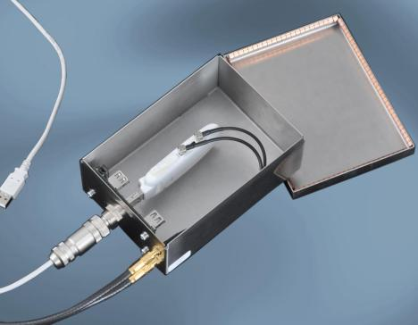
RF Guard is employed in wireless network test labs to protect USB controlled handsets, modems and data sticks from any undesired RF interference. Only the radio signal from an (e)NodeB, a base station or a network simulator is supplied to the terminal inside the shielding box. Two RF inputs ensure compatibility with MIMO equipment. USB 2.0 ports provide for power, voice and data exchange with the enclosed terminal.
