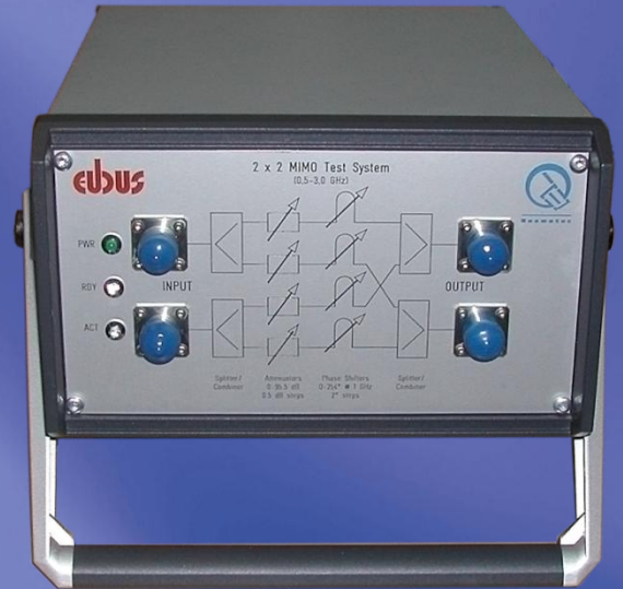
AIS 2x2 MIMO portable unit with phase shifters
